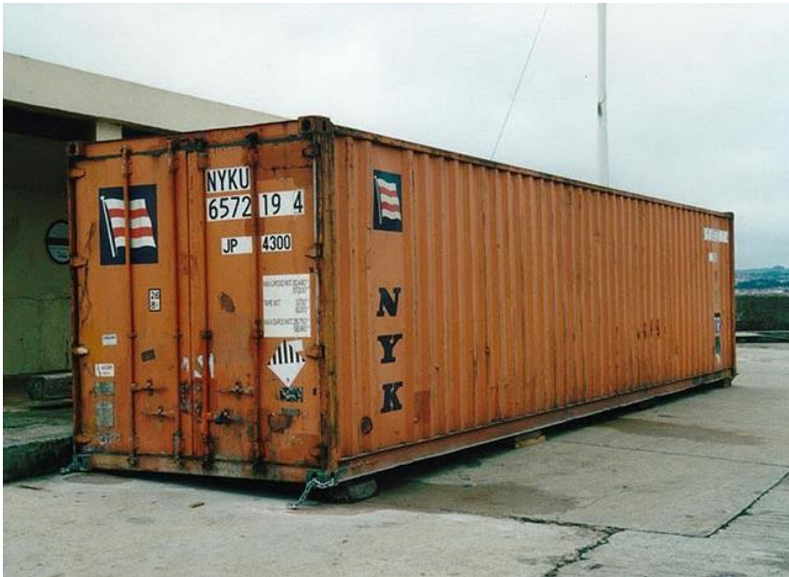
Figure 2.2: A typical 40' ISO global shipping container
