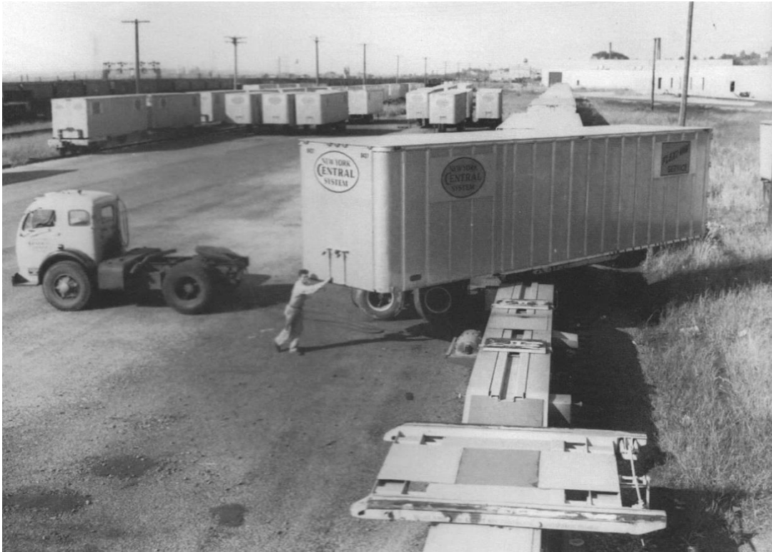
Figure 5.3: Flexi-Van container being moved between truck and railcar
