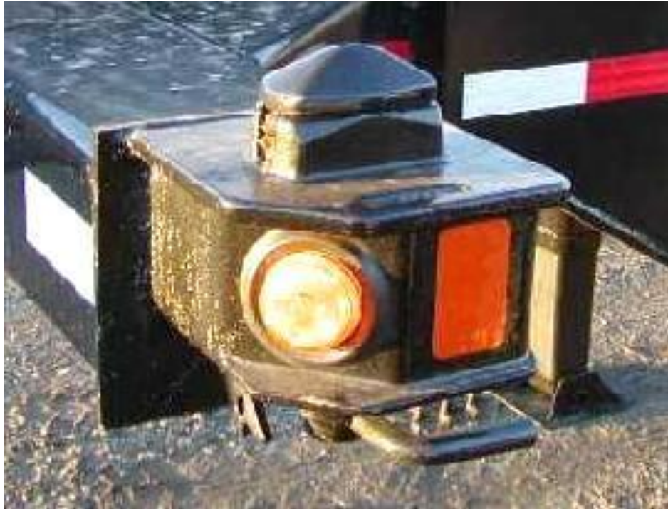
Figure 6.2: Twistlock on a trailer chassis
