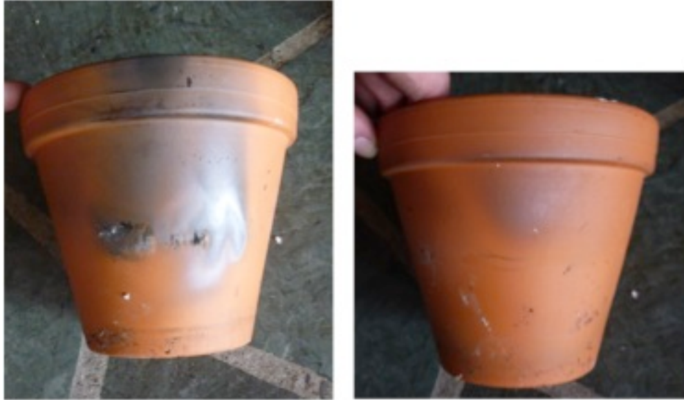
Figure 183. Large flower pot is not blackened below where charcoal sat (see pencil line)
