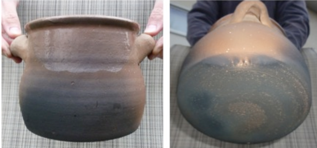
Figure 179. Soot on pot immediately after Test 2
