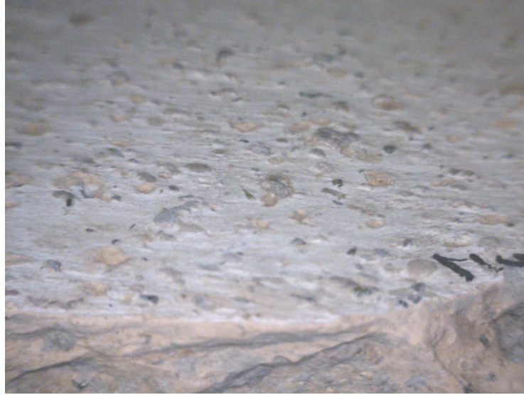
Figure 128. Pedestalling visible on mortarium surface at 20x magnification (MUS 850)
