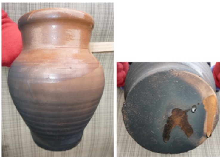
Figure 176. Sooting on pot immediately after Test 1
