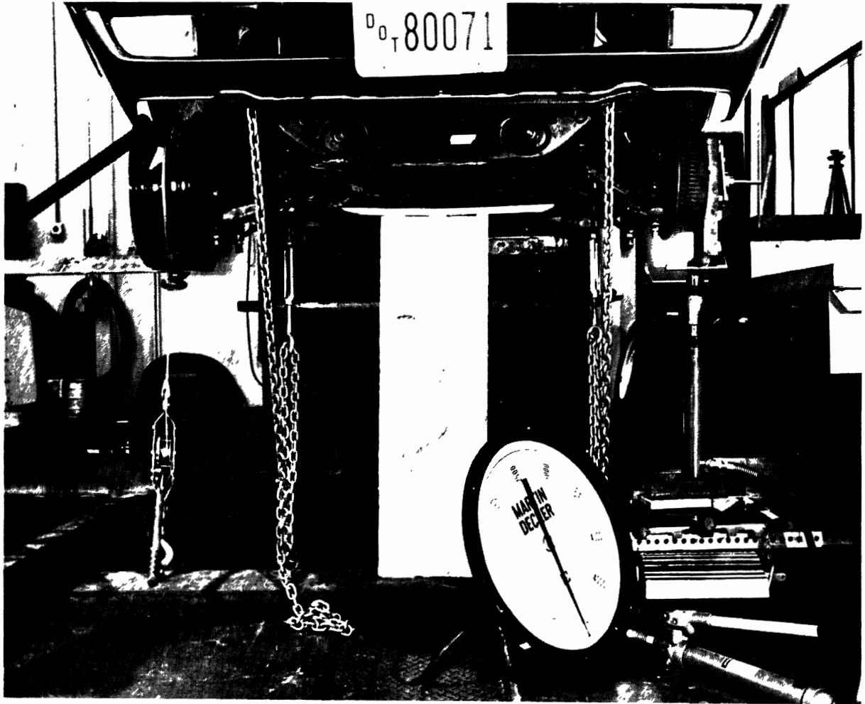
Figure 3.4. Setup for measurement of suspension properties
