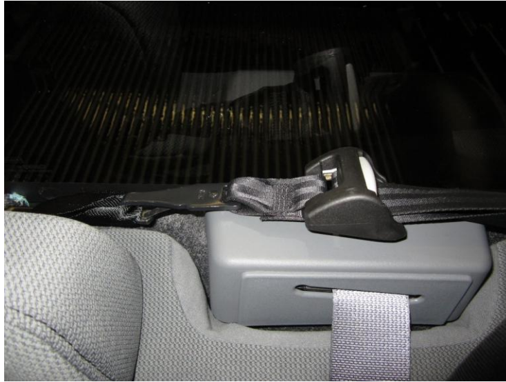
Figure 30. Triumph tether adjuster hardware does not fit behind seatbelt mount as directed.
