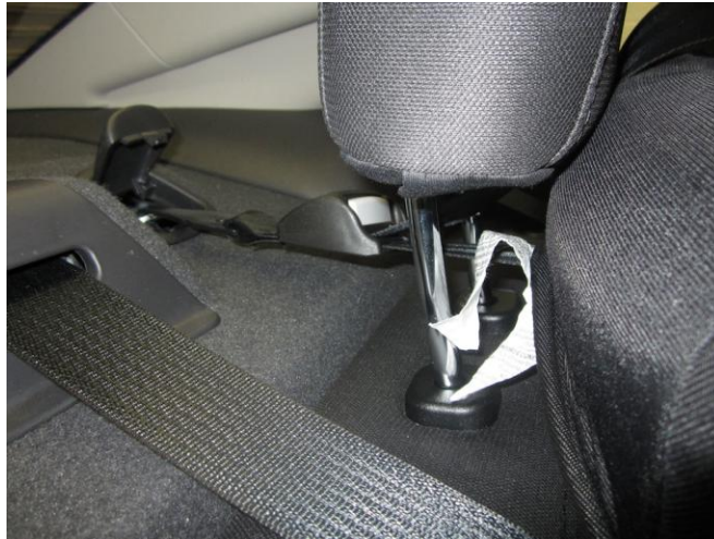
Figure 27. Example of subjects leaving the head restraint in non-locked up position against manufacturer directions.
