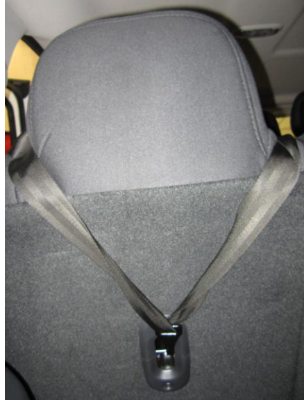
Figure 31. Method used by all subjects to route the V-style tether (when used) on the Jeep Patriot.
