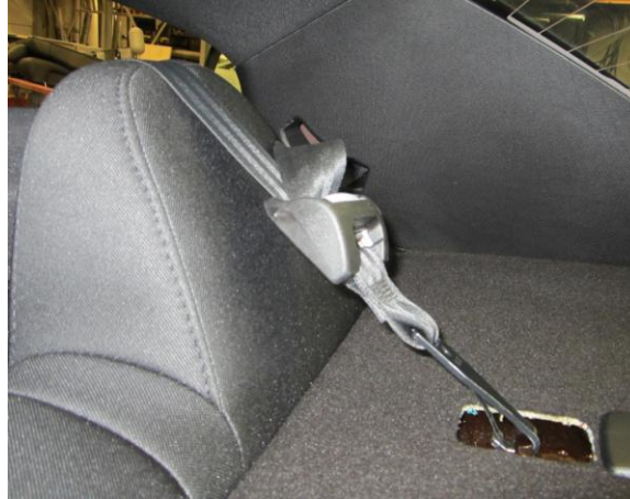
Figure 32. Some subjects incorrectly routed the tether over the top of the head restraint rather than outboard of the head restraint.
