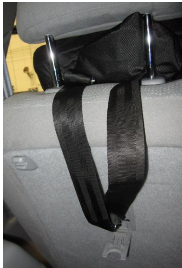
Figure 23. Example of V-style tether being slightly pinched when routed under head restraint as directed, as well as interference between CRS and head restraint.
