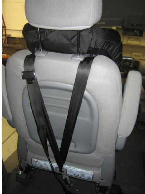
Figure 25. Example of subjects routing Marathon tether around head restraint posts.
