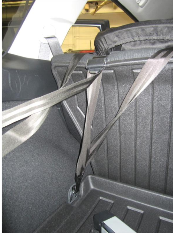
Figure 26. Example of subjects incorrectly attaching tether to cargo tiedown.
