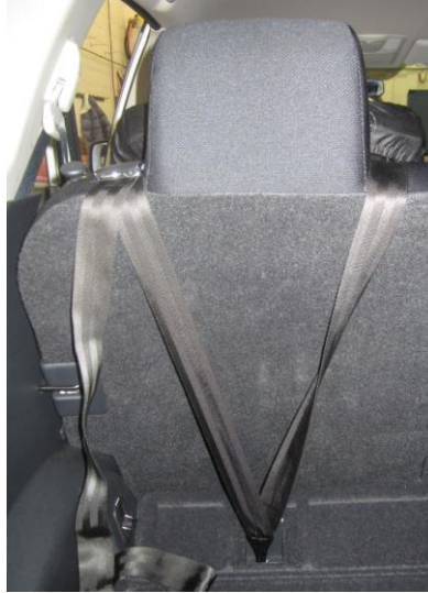
Figure 22. Most subjects routed the V-style tether around the head restraint rather than over.
