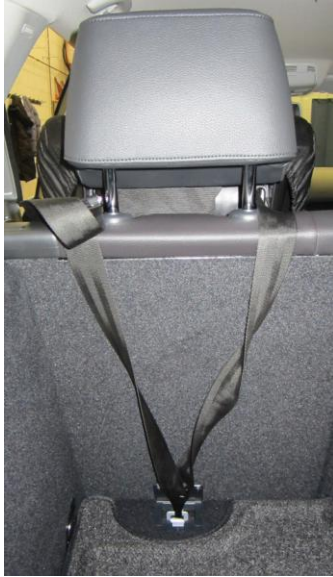
Figure 33. Subjects often routed V-style tether around the head restraint posts rather than in between.
