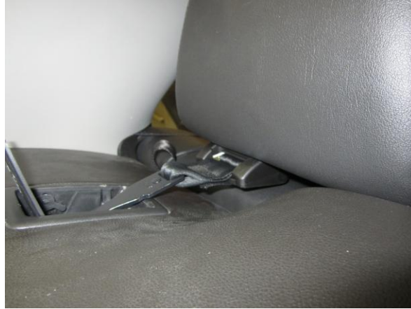
Figure 29. Example of tether adjustment hardware interfering with proper positioning of head restraint.
