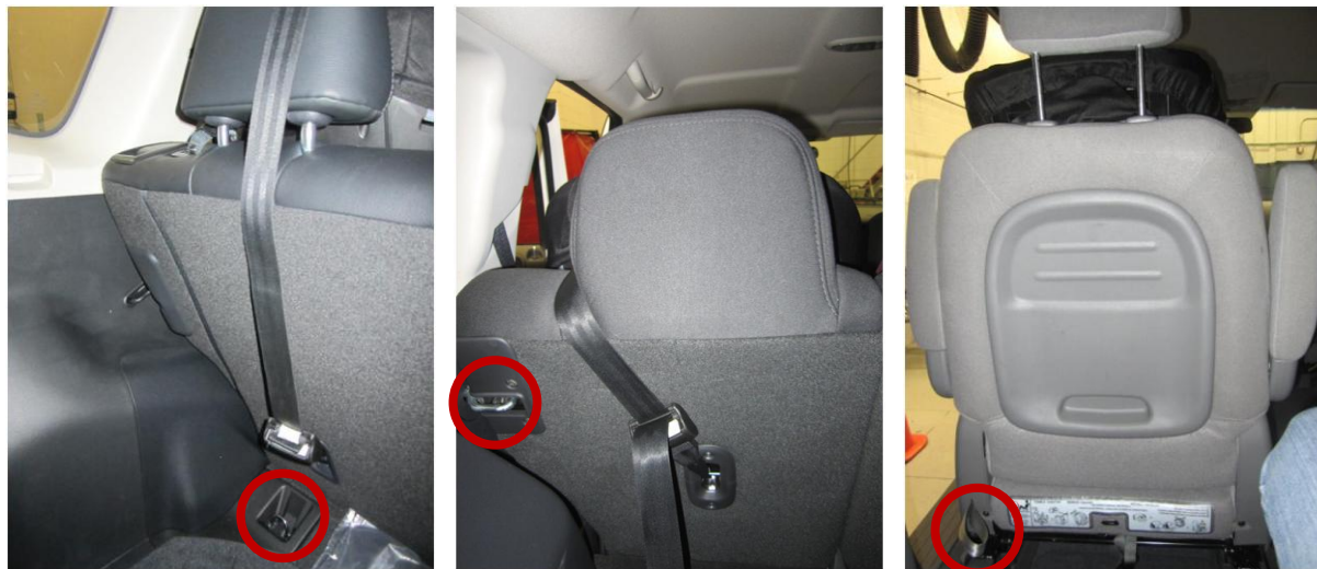
Figure 6. Potentially confusing hardware includes cargo tie-down points (left and center) and webbing loops (right).
