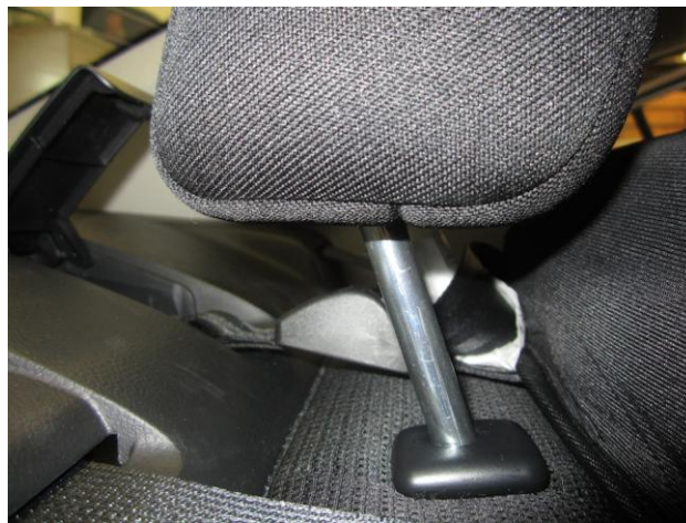
Figure 20. Tether adjuster ends up underneath HR, making it difficult to tighten.
