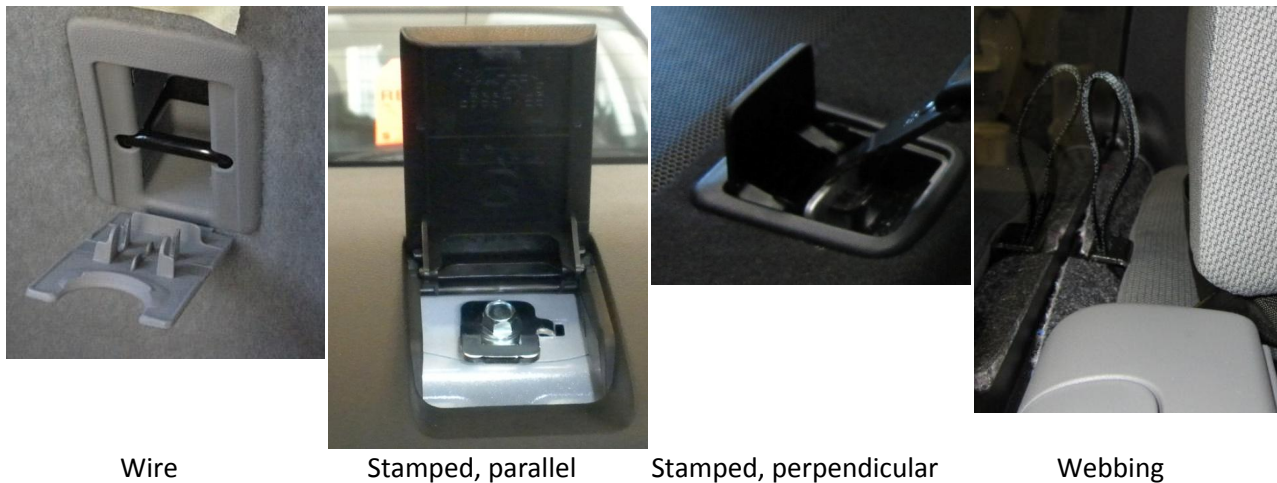
Figure 4. Different categories of tether construction.
