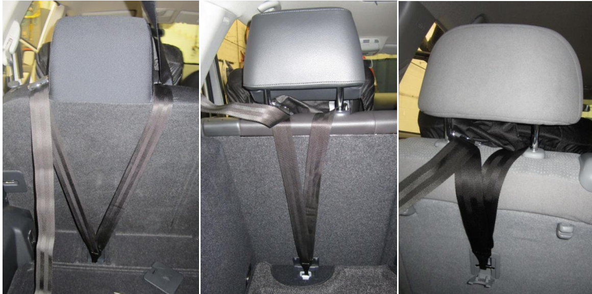
Figure 34. Location of adjuster for V-style tether varies with the height of the vehicle seatback.
