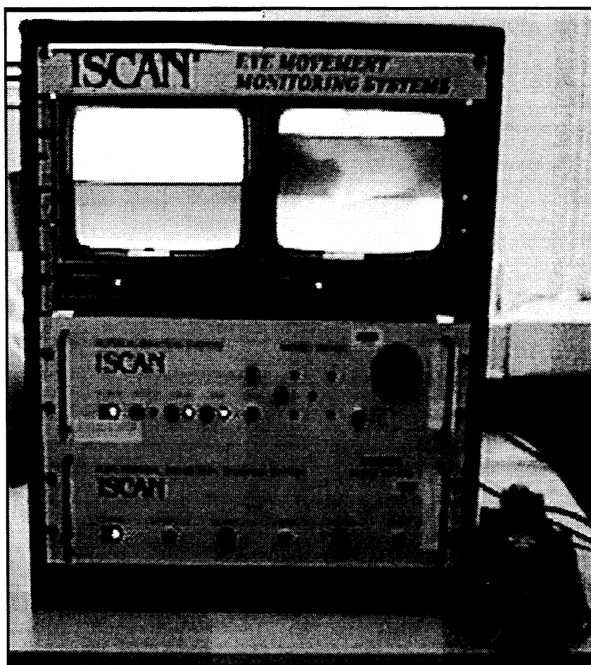
Figure 14. The control panel for the ISCAN.
