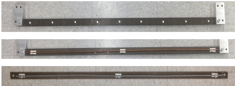
Figure 11. Test Specimens: front view(top), specimen 1(middle), and 2(bottom)
