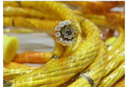
Figure 1. Helically twisted 1x18 space flight cable used for experimental testing.
