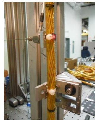
Figure 4. Cable attachment point and driving point.
