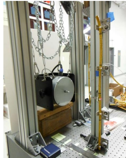
Figure 3. Testing of space flight cable with pinned end conditions, suspended shaker, and load cell force input in controllable environment.
