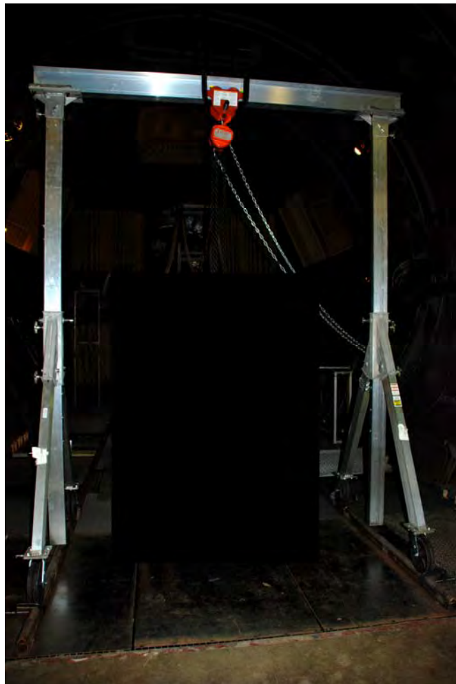
Figure 4.27. Photograph of gantry crane on the portion of the rail system that extends onto the flat paneled grating of Figure 4.26.
