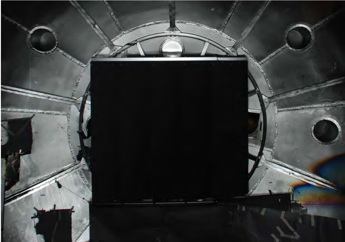
Figure 4.32. PEPL LVTF graphite beam dump mounted on the endcap.
