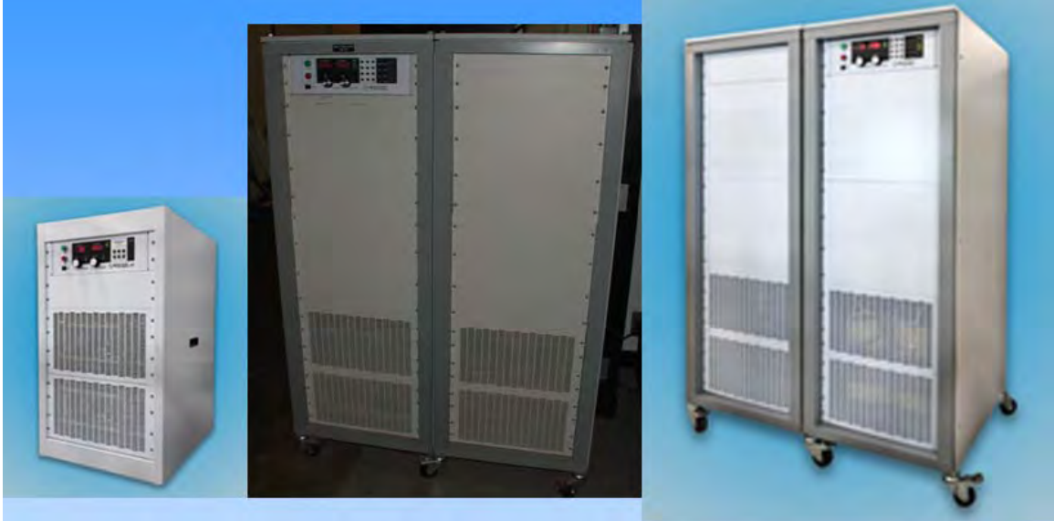
Figure 4.2. The three discharge power supplies for the X3 (left-to-right): 60 kW (Magnapower MSD1000-60/480), 100 kW (Amrel HPS1000-100), and 150kW (Magnapower MTD1000-150/480).
