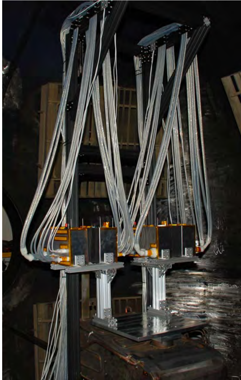
Figure 4.8. PEPL's universal waterfall, sans thruster. The boxes which accept the wires from the flange are not pictured here.
