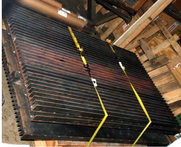
Figure 4.26. Steel grating required to bridge the gap between concrete floor outside LVTF and interior grating (stowed in this picture). Each unit weighs over 45 kg.
