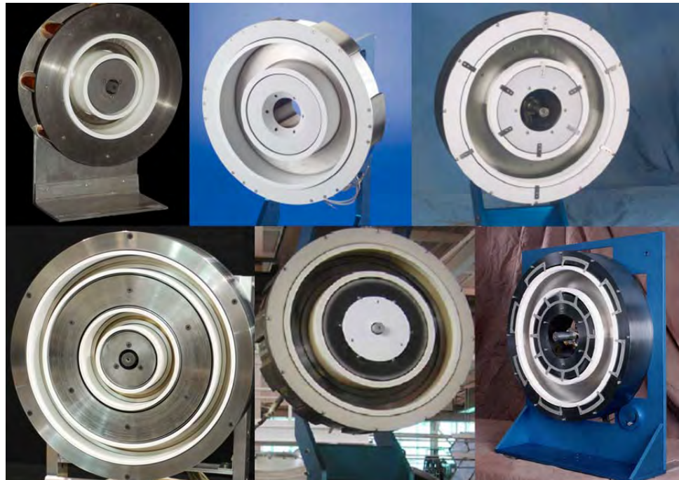
Figure 2.3. The family of thrusters that influenced the X3, CW from top Left,; H6, 75 NASA-300M, 76 NASA-400M, 77 NASA-457Mv1, 24 NASA-457Mv2, 78 X2 NHT. 9
