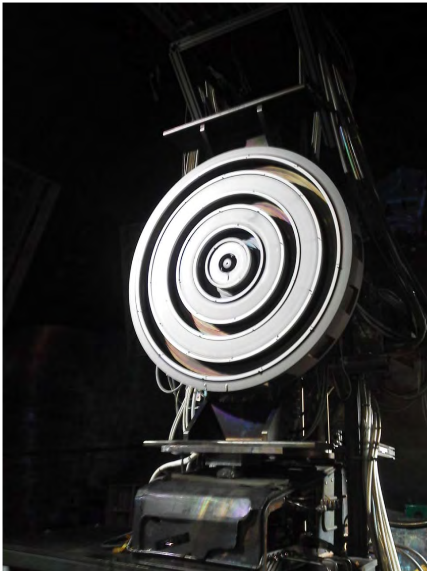
Figure 4.29. The X3 mounted on the thrust stand in LVTF.
