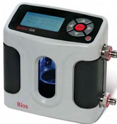
Figure 4.15. Bios Definer MFC calibration unit Low- and mid-range units are identical in appearance except for a different sized piston. Hence only one unit is shown here. 88
