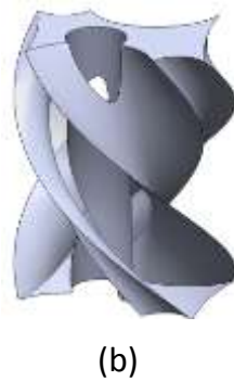
Figure 4.2 CAD of T-junction that funnels CA and SBF into a single entry pathway towards vascular phantom. CAD of the inverse of the T-junction with inline fluid mixer positioned downstream of the T-junction outlet. (b) Single unit of the helical mixer (complete mixer composed of 6 repeating units).
