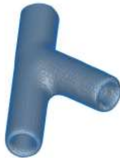
Figure 2.5 CAD of three-dimensional triangulated surface mesh for a first order bifurcating tree.
