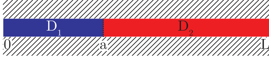
Figure 7.1: One dimensional heat conduction problem domain. Phase 1 is the blue region with diffusivity D_1 , and phase 2 is the red region with diffusivity D_2 . The rod is insulated along its length, which only allows for heat conduction across the endpoints.
