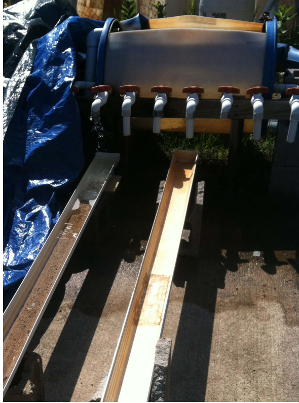
Figure 4.2: Header tank, taps, and two channels for the NUS Team's artificial stream setup.
