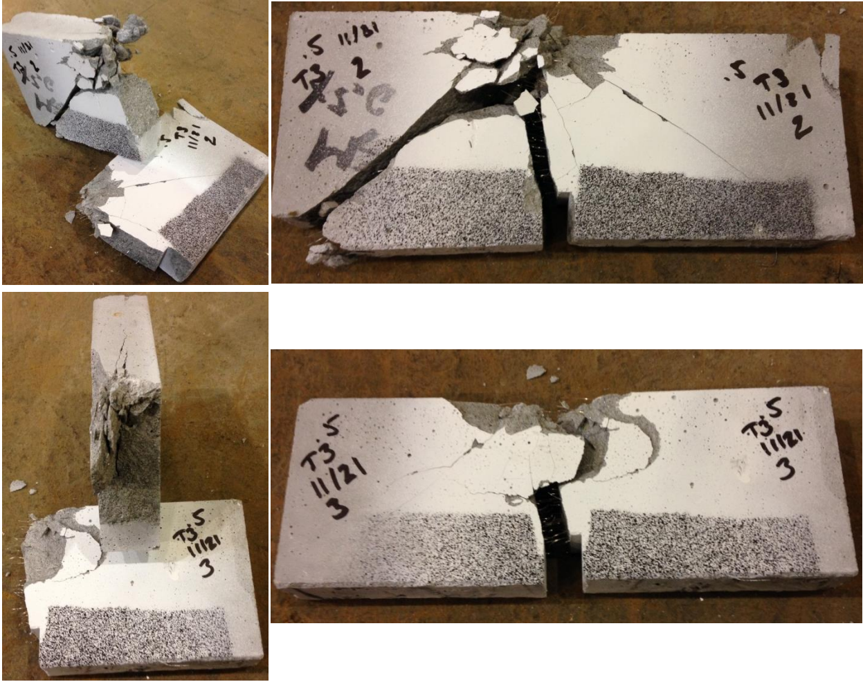
Figure 6.20. Examples of CS-0.5% specimens with crushing failure tested in M-SEFIM with Type 3 coupler
