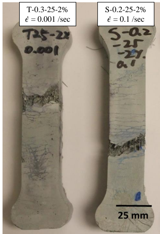
Figure 3.15. Representative multiple cracking patterns in UHP-FRC specimens
