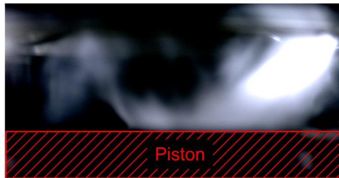
Figure 6-12. Unprocessed still image of the fuel spray at 310 °bTDC (10 CAD after SOI) for E100 with SOI = 320 °bTDC and T_{\text{coolant}} = 90\text{ °C} .
