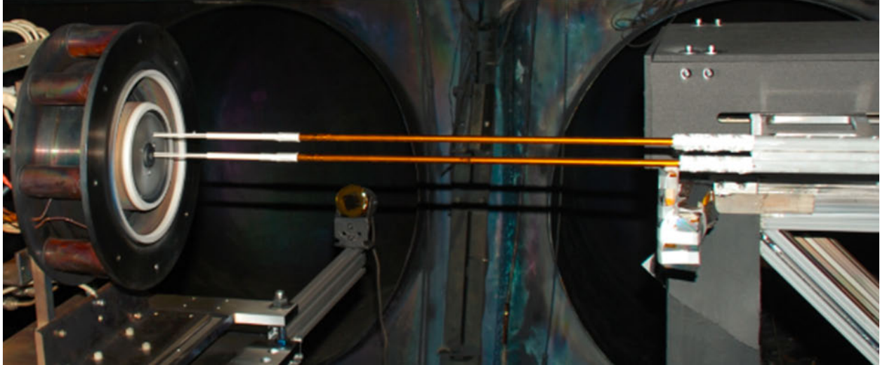
Figure 3.1: HDLP-ISR mounted on HARP shown at full extension to the discharge channel exit plane ( z/R_{chnl} = 0 ) on cathode centerline ( r/R_{chnl} = 0 ). Note the ISR probe is over the outer pole. This configuration was used to generate the plume maps in Appendix B.
