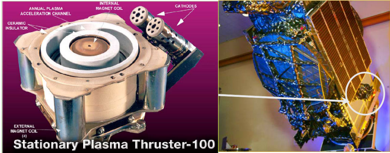
Figure 2.1: SPT-100 with key components and typical mounting on Space Systems/Loral spacecraft. Primary use on SS/L communication satellites is for north-south station keeping. Reproduced from Figure 1 of Ref. 19.
