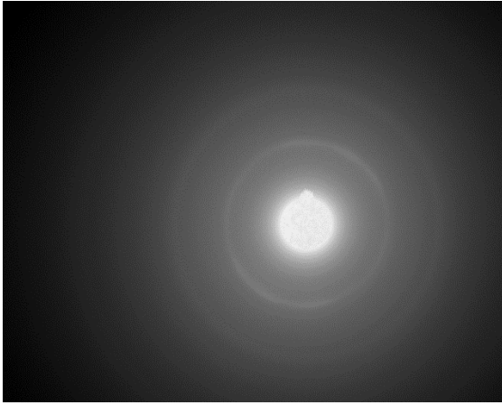
Figure C.14. Diffraction pattern 37 recorded for the sample irradiated at 1000°C 20MPa to 1.0dpa.
