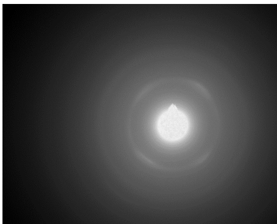
Figure C.9. Diffraction patterns 7-12 recorded for the sample irradiated at 1000°C 20MPa to 1.0dpa.
