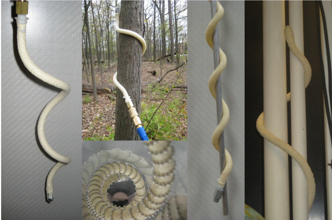
Figure 6.8: Helical FREEs demonstrating helical shape generation, rough object grasping, small object grasping, asymmetric object grasping, and pipe anchoring.
