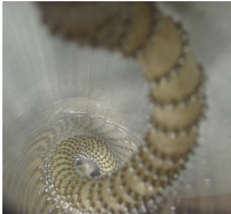
Figure 6.10: Helical FREE pipe inspection device is inflated in a 2.25 inch inner diameter clear pipe, viewed inside the pipe. The device has fiber angles of 88^\circ and -80^\circ for the families of fibers and 5^\circ for the single fiber.
