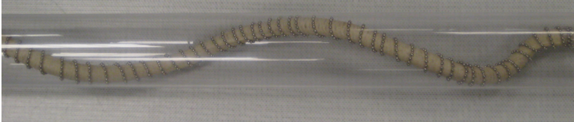
Figure 6.9: Helical FREE pipe inspection device is inflated in a 2.25 inch inner diameter clear pipe, viewed from the side. The device has fiber angles of 88^\circ and -80^\circ for the families of fibers and 5^\circ for the single fiber.
