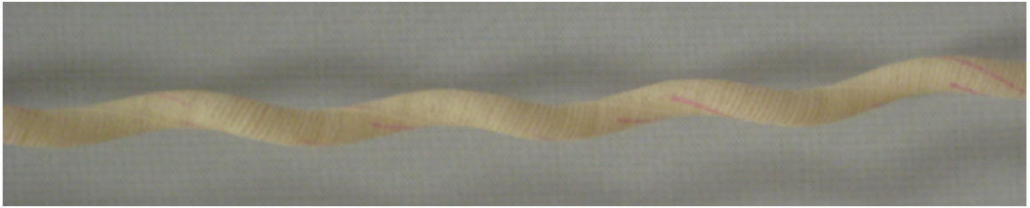
Figure 6.5: Helical FREE with \alpha = -70^\circ , \beta = -30^\circ , and \gamma = 1^\circ . The helical FREE prototype has a body radius of 6 mm and was inflated to a volume increase of 35%. The image is the inflated helical FREE (image rotated 90 degrees, gravity going right).
