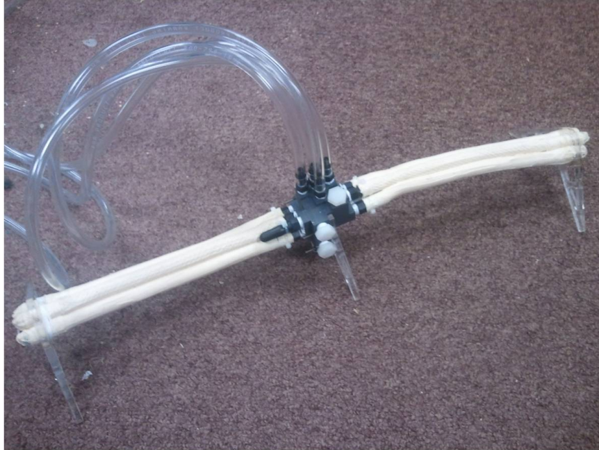
Figure 5.9: Hexapod robot with a parallel FREE spine that generates a walking gait through selective pressurization of individual FREEs.
