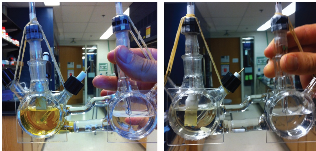
Figure 3.18 Images of PEC cells after j - t experiment using \text{WO}_3 (left) and \text{CuWO}_4 (right) in buffer containing \text{Cl}^- . The \text{WO}_3 experiment was conducted in pH 5 solution containing 0.1 M NaCl and the \text{CuWO}_4 experiment was conducted in a 0.1 M \text{KB}_i buffer containing 0.1 M NaCl.
