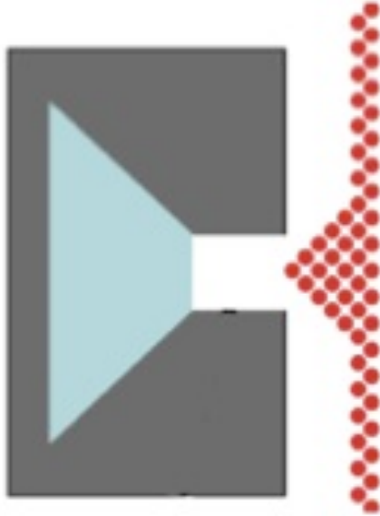
Figure 1.1: Depiction of Virtual Cathode Effect due to Single Polarity Emission
