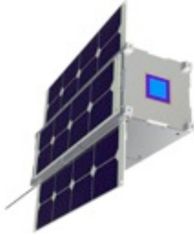
Figure 1.6: Depiction of the NanoFET System (in blue) on a Single Side of a 3U Cubesat ( Liu, 2010 )
