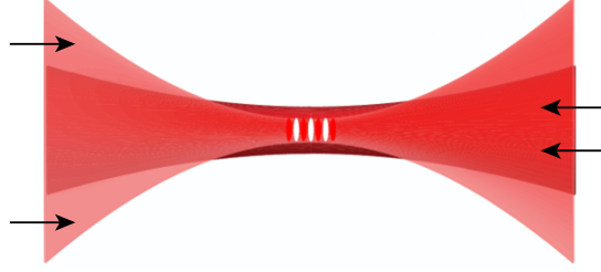
Figure 7.1: Laser beam diagram for a three-dimensional bottle trap for Rydberg atoms. The foci and powers of the two counter-propagating lattice beams are adjusted to achieve intensity matching on-axis, surrounded by a non-zero light field.
