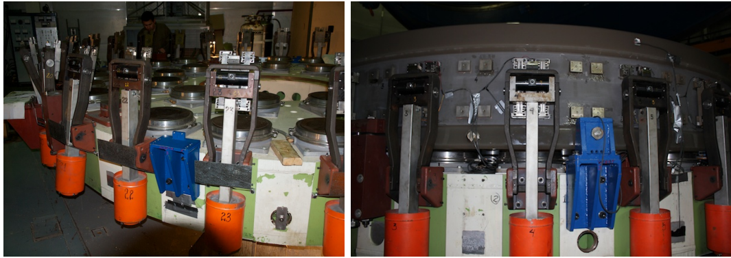
(a) Mirror cell for primary mirror (b) Mirror cell with primary mirror mounted
