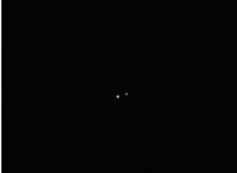
Figure A.2: A typical image taken using a BCAM. The BCAM which flashed its lasers in this image did so for 0.6 ms per laser, for a total exposure time of 1.2 ms. The separation between the lasing and imaging BCAMs in this pair is approximately 10 m, as measured along the line-of-sight between them. The image contrast was increased to show the spots more clearly.
