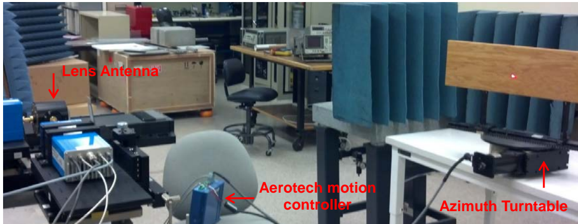
Figure 6.16 The backscatter measurements setup. The sample distance to the antenna is 2 meters.
