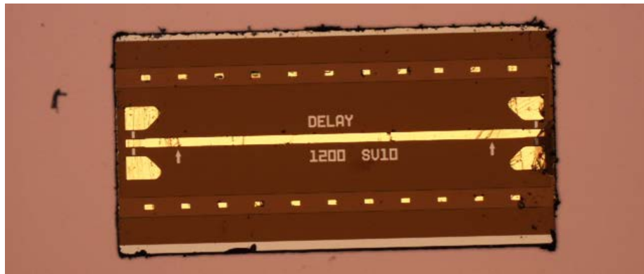
Figure 4.13 Delay lines implemented on 55 \mu\text{m} thick InP with the old launch pad design
