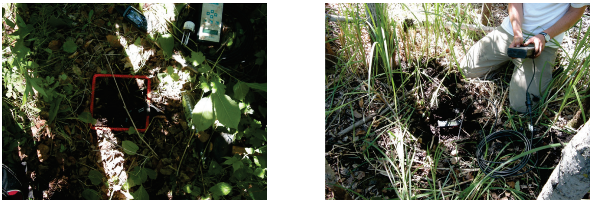
Figure A.5: Soil moisture sampling location (left) with inserted soil moisture probe (right).
