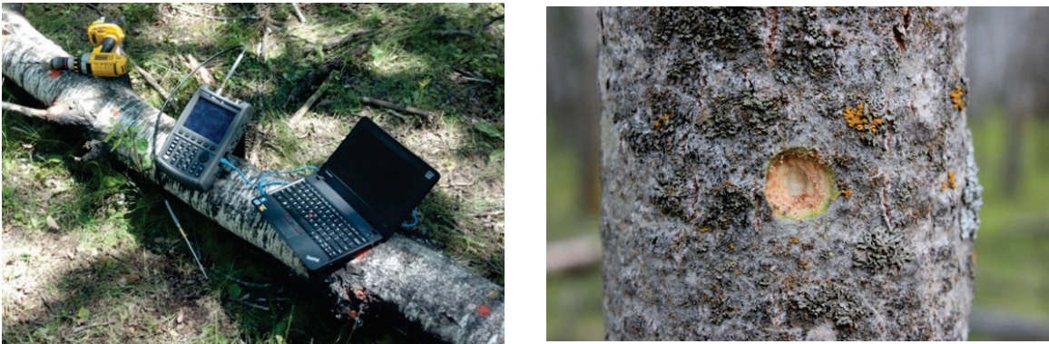
Figure A.13: Example setup with FieldFox and laptop (on left) and drilled hole to be probed (on right).
