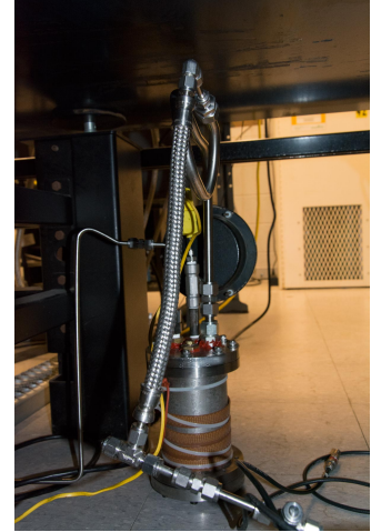
(c) Back view of acetone bubbler with tubing connected.
