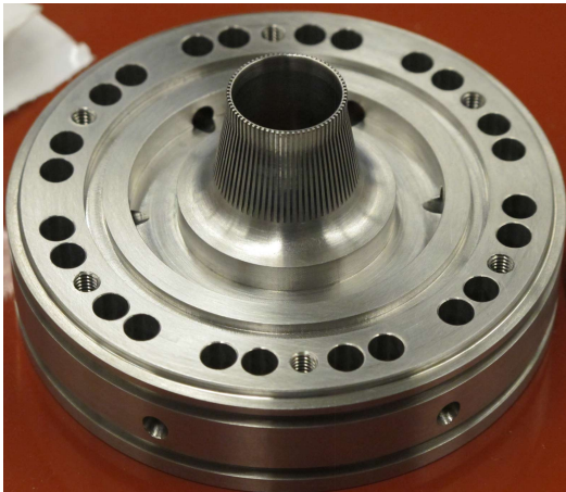
(b) View of the GTMC inner air nozzle and fuel channels.
