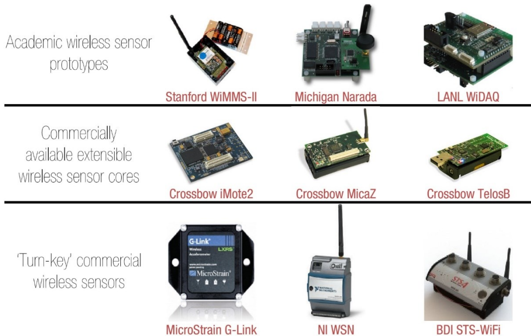
Figure 2.20 Wireless sensor families and selected examples (G-Link photo courtesy of LORD-MicroStrain, NI WSN photo courtesy of National Instruments and BDI STS-WiFi photo courtesy Bridge Diagnostics)
