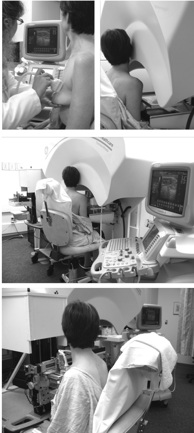
Fig 5.1: Pictorial representation of the progression of experiments conducted during a typical human subject scan in this study. Top left: First, a radiologist conducts a direct contact hand scan to initially localize the breast mass and compare image quality with through-paddle ultrasound scan. Top right: Subject's breast is compressed in the combined tomosynthesis/ultrasound system for acquisition of x-ray tomosynthesis images. Middle: While the breast is still compressed, the ultrasound transducer is scanned across the entire breast to obtain a full-field 3D volume of the breast in the same orientation and at essentially the same time as the tomosynthesis image. Bottom: The subject is moved from the combined system to the stand alone mammography-mimicking unit for precisely controlled through-paddle elastography.
