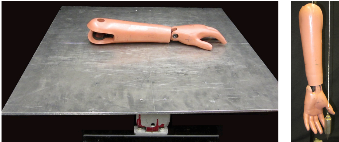
Figure 3. Balance table (left) and hanging (right) methods for measuring limb segment center of mass.
