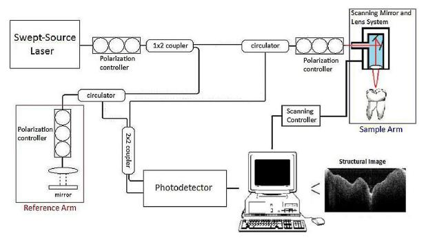
Fig. 1. OCT System setup.
