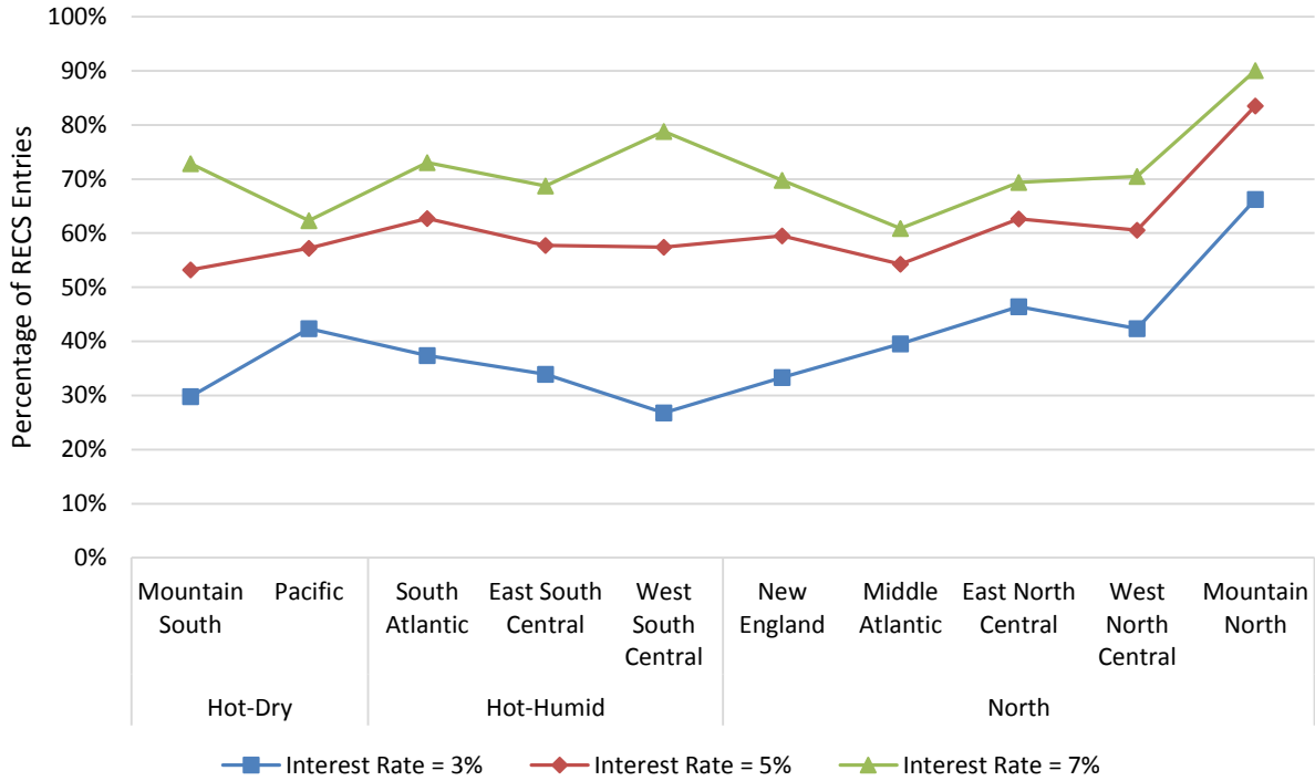
Figure 43. Percentage of RECS entries where GHP system is more expensive than conventional system. Note that interest rates play an important role in evaluating the economic performance of the GHP system.
