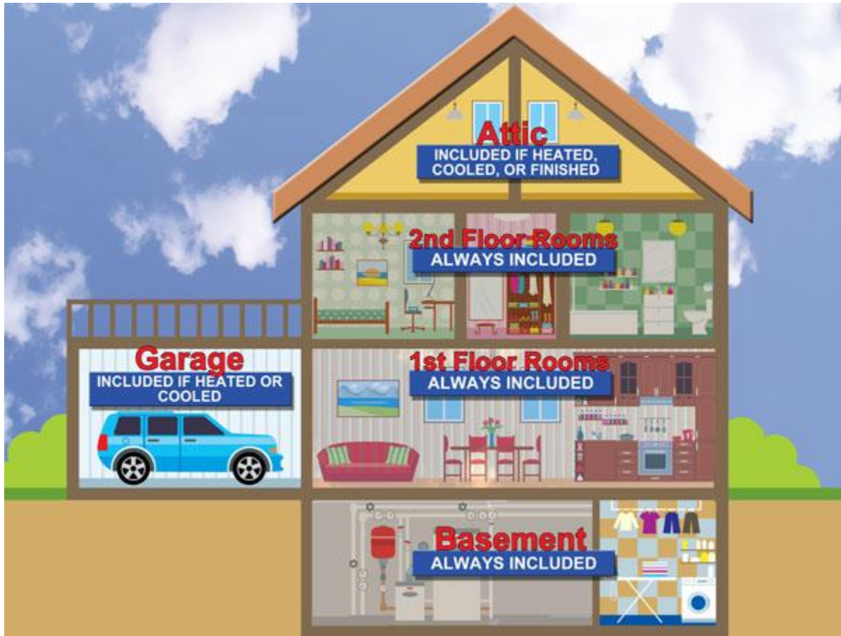
Figure 23. Graphical description of how house square footage is calculated in the RECS 2009 dataset. See Error! Reference source not found. for total square footage of a house. The square footage of the house is measured by the interviewers during the survey. EIA performed in-person measurements as many alternative sources such as property tax records, real estate listings, and respondent estimates use varying definitions which underestimated house square footage for the purpose of energy analysis 1 .
