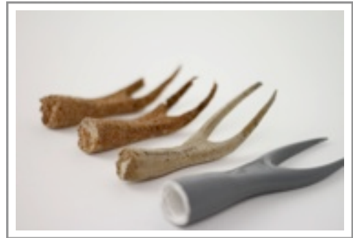
Figure 16- Trial models of the version 1 Temp Tool roaster using a plastic mold
