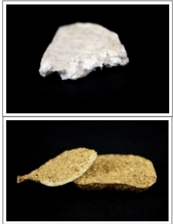
Figure 13 and Fig. 14- View top: first material test, gelatin glue and paper pulp. Seen bottom: final material selection, gelatin glue and wood sawdust
