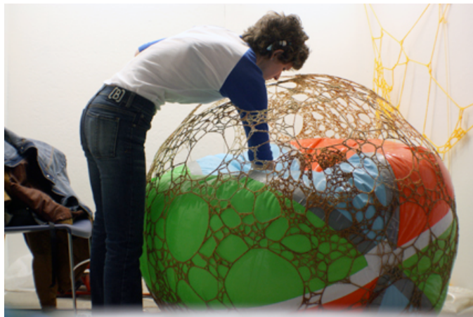
Fig. 1 – Deflating the supporting structure after glue has been applied and cured.
