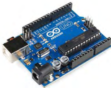
Figure 15- Arduino Uno board (image taken from www.sparkfun.com ).
