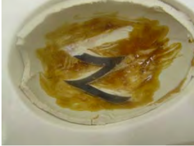
Figure 14- Area applied with Shellac will resist water and, thus, not rub away with a wet sponge.
