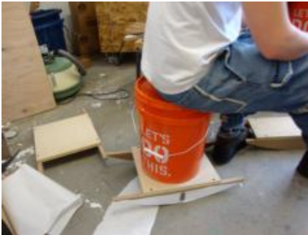
Figure 5: Testing a variety of radii for the bottom of the active-seating stool (or rocking stool). I found that, for someone of my height, a 25” radius caused too much rocking and motion sickness, whereas 27.5” did not provide enough motion. The compromise, 26.25”, worked very well.
