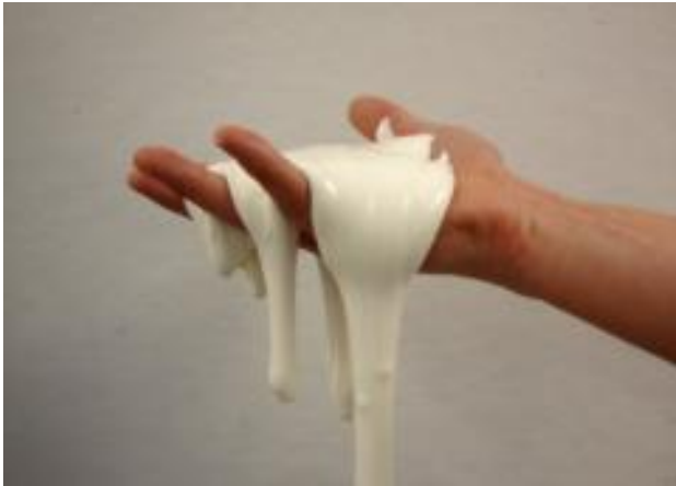
Figure 3: The non-newtonian fluid I developed consisting of white glue, cornstarch, water, and borax. It can crumble like feta cheese, but oozes to the ground when there is no pressure.
