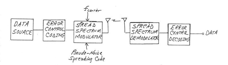
Figure 1 Spread Spectrum Concept
