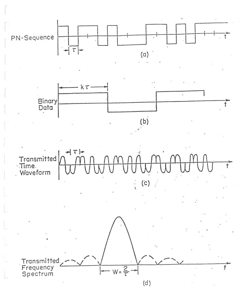
Figure 3 Frequency Hopping (FH) Systems PN Sequence used as a Random Number Generator
