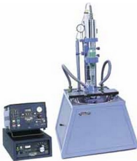
Figure 2.1 : Sonic-Mill® AP-1000 ultrasonic machine [Son14a]
