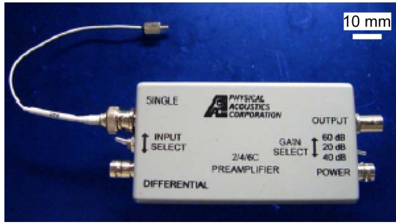
Figure 2.4: HD15 acoustic emission sensor with 2/4/6C preamp from Physical Acoustics Corporation [Li09].
