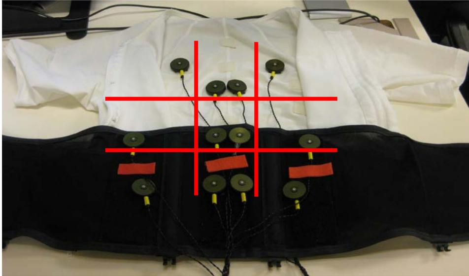
*Figure 3-2: Tactor vest (top, Veronique brand) and belt (bottom) divided into nine sectors to map onto the nine UAV feeds on the monitor*
