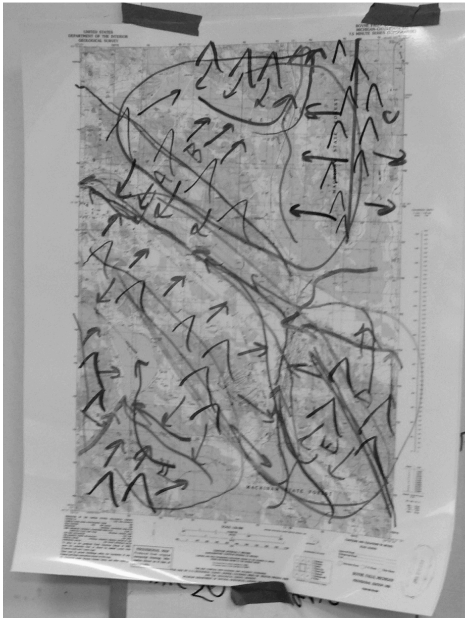
Figure 6. The annotated map showing the paths of the water and the paths of water drops A through F. Lighter colored lines indicate dividing lines created by the areas of high elevation.
