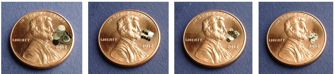
Design A Design B Design C Design D Ø2 mm discs Ø0.985 mm discs Ø0.4-1 mm rings Ø0.2-0.5 mm rings
