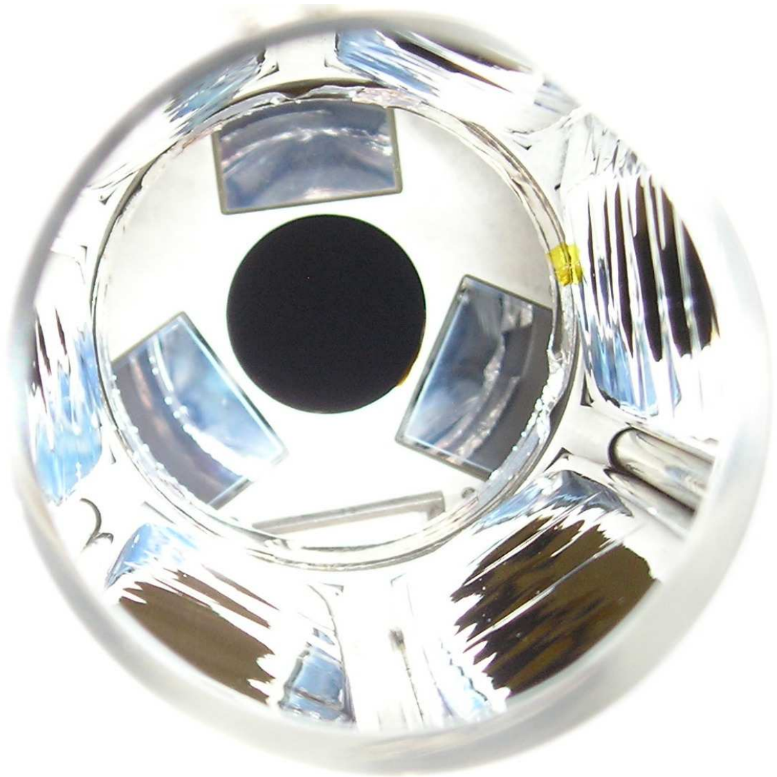
Figure 2.15: Photo of version 2 of the LAAPD detector array, which was present during approximately one third of RDK II's operation. This view is shown in the direction that is upstream of the neutron beam. The three LAAPDs are partially visible. The aluminized Mylar wrap around the BGO detector array can be seen at the edges of the photo. All data presented in this dissertation was taken using this version of the apparatus.
