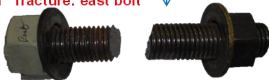
Figure 6.76 Photographs of Bearing PB13 taken during and after cyclic loading
