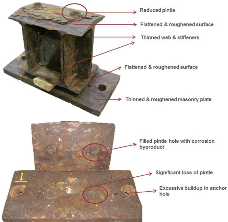
Figure 5.1 Illustration of various corrosion locations and effects on a steel rocker bearing salvaged from an abutment
