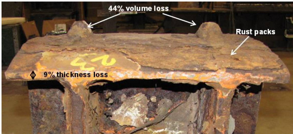
Figure 6.54 Top cylindrical surface of Bearing AR23 in the as-received condition
