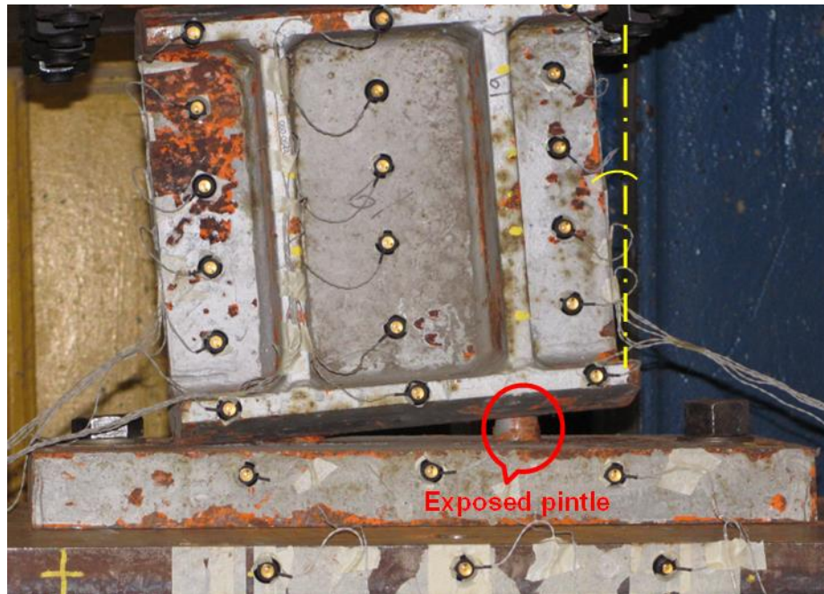
Figure 6.34 Photographs during testing of Bearing PR19 under transverse monotonic loading
