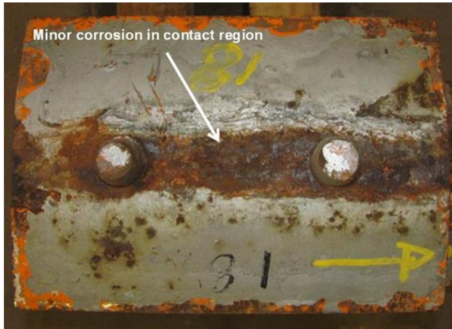
Figure 6.27 Top cylindrical contact surface of Bearing PR18
