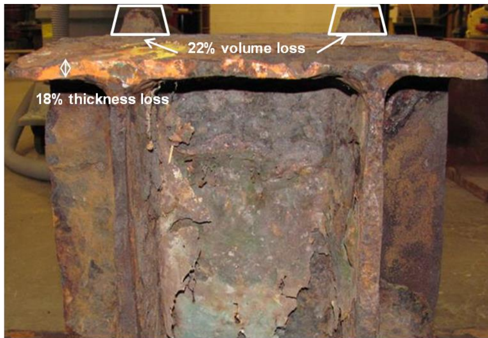
Figure 6.18 Abutment rocker bearing #25 (AR25) in its as-received condition
