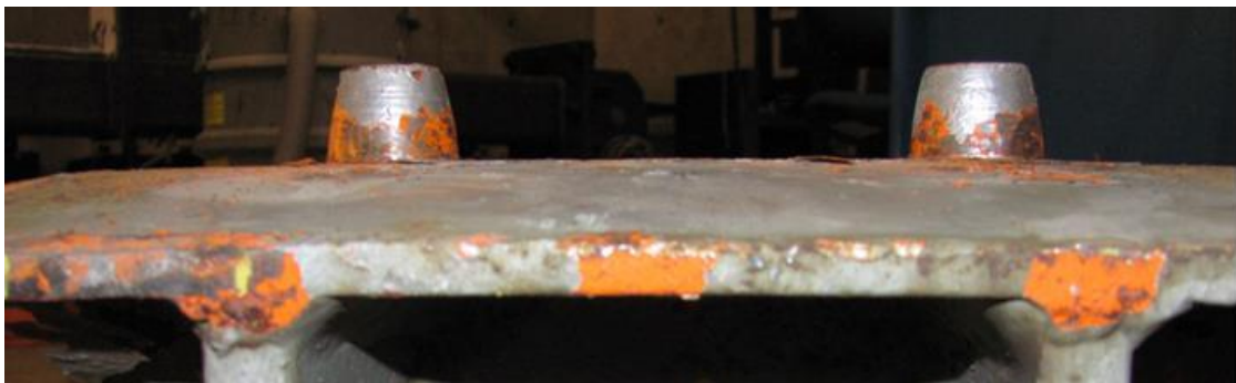
Figure 6.75 Top contact surface with pintles of Bearing PB13 in the as-received condition
