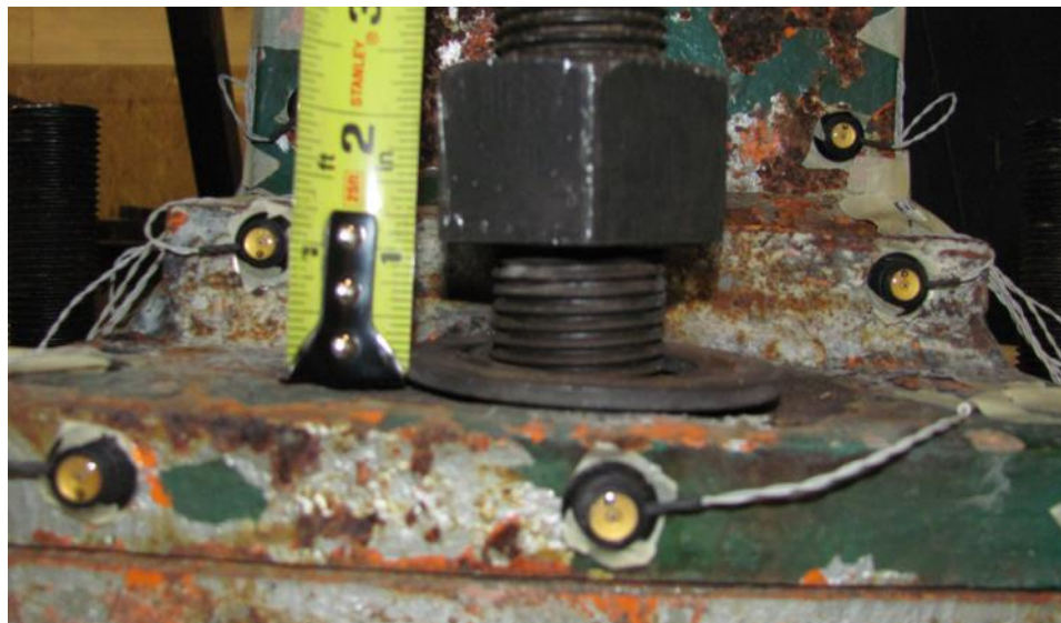
Figure 6.94 Photographs showing bolt pullout and bearing rocking behavior
