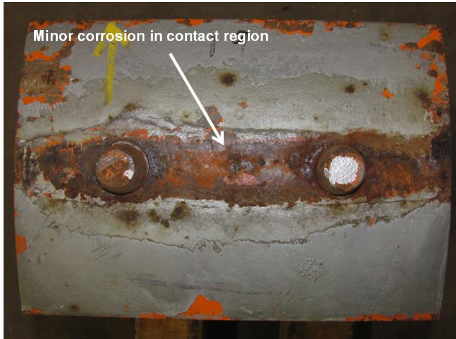
Figure 6.32 Top cylindrical contact surface of Bearing PR19
