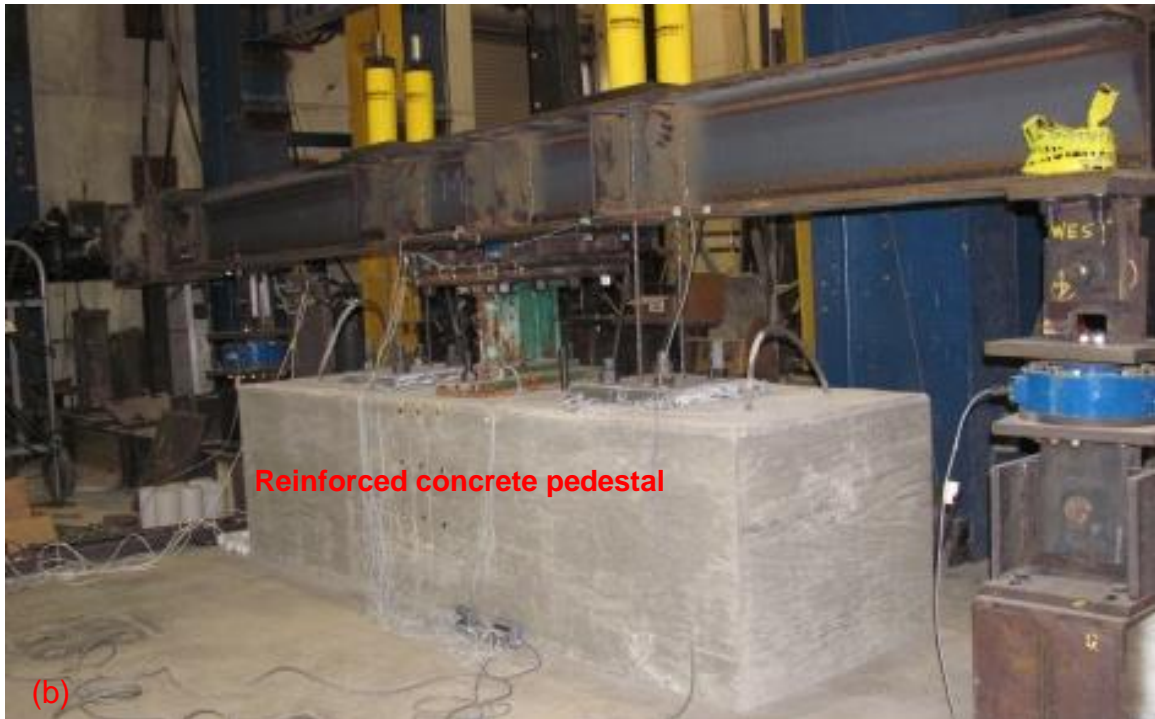
Figure 6.2 Photograph of the bearing test setup
