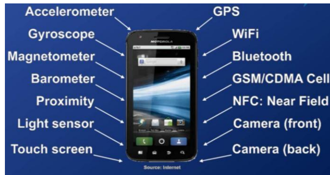
Figure 1.2. Diversified functions integrated in a typical user-end terminal, including wireless communications and sensors.
