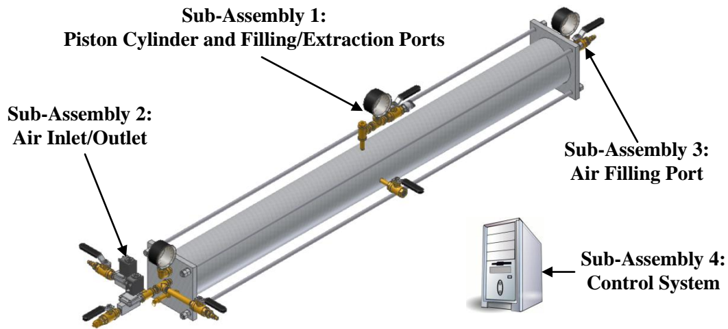
Figure 8.3: Four main sub-assemblies of final design
