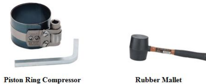
Figure 9.36: Piston cylinder installation tools
