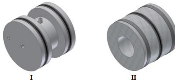
Figure 9.23: Concept piston (I) and reference piston (II) final assembly
