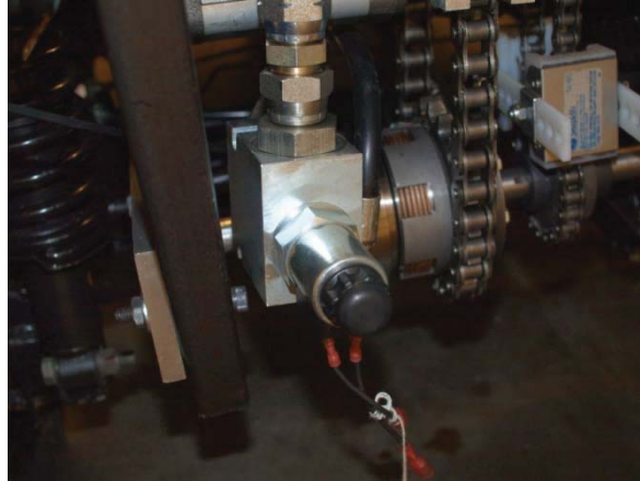
Figure 2. Faulty recirculation valve currently installed on the vehicle
