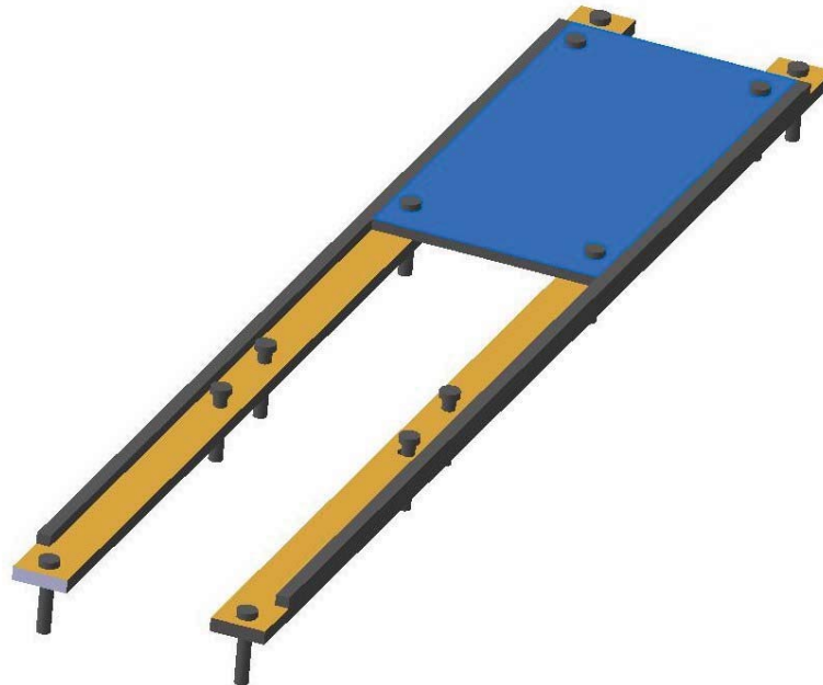
Figure 16: Final mounting mechanism for slow fill pump, manifold, and filter
