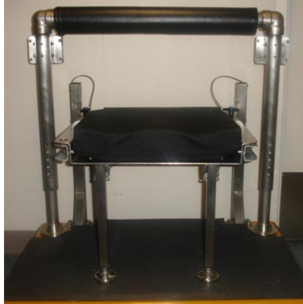
Figure 2: Seat design from surgical lift from Fall 2008 ME 450 team
