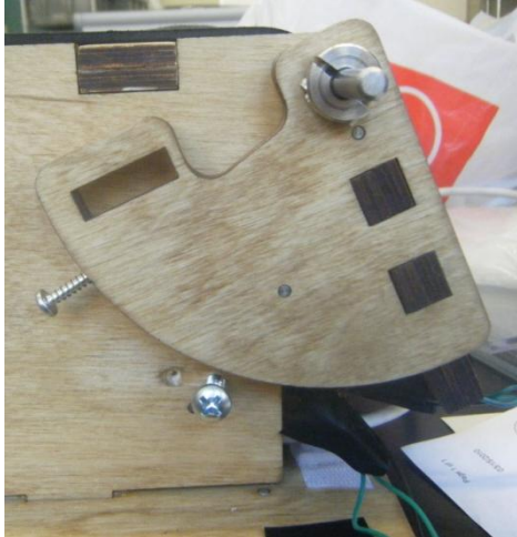
Figure 35: Mechanical stop in disengaged position
