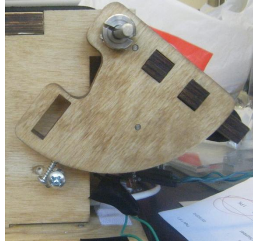
Figure 36: Mechanical stop mechanism in engaged position
