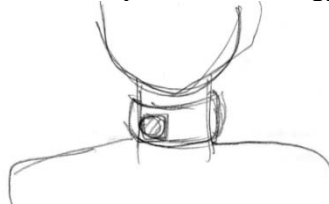
Figure D.2: Piezoelectric throat strap to collect energy from human vocal cord
