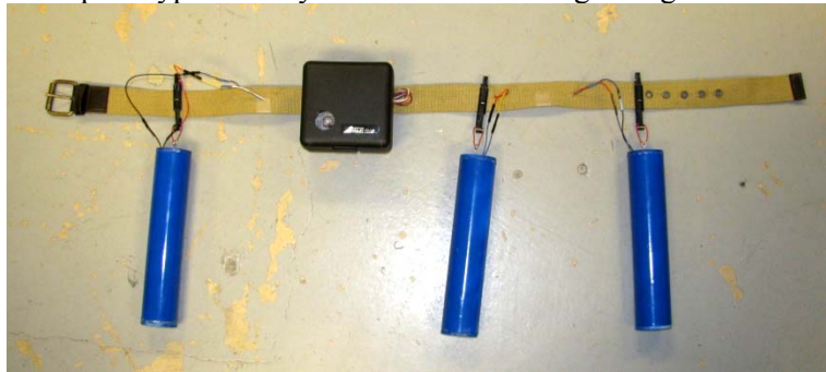
Figure 11.1: Final prototype - belt system with electromagnetic generators and a black box
