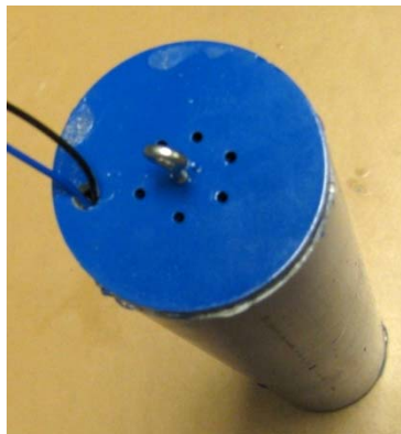
Figure 11.3: Cap of the canister has holes for air flow and eyelets for spring and ALICE clip attachment
