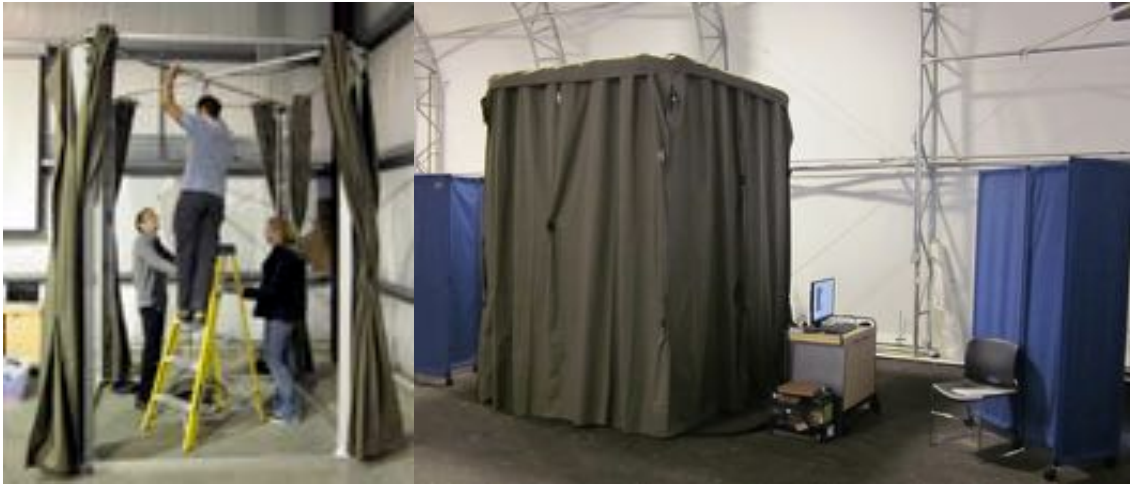
Figure 16. Investigators setting up the four columns of the Human Solutions Vitus SSL scanner (left), and the scanner set up at Fort Hood (right).
