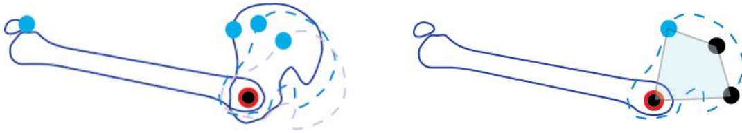
Figure E12. Digitizing knee and ASIS (in different postures) in vehicle seat and then using the knee-hip length and ASIS-hip length to calculate the hip joint location (left) and then using the ASIS and hip joint to calculate the lower lumbar joint and PSIS locations (right)
