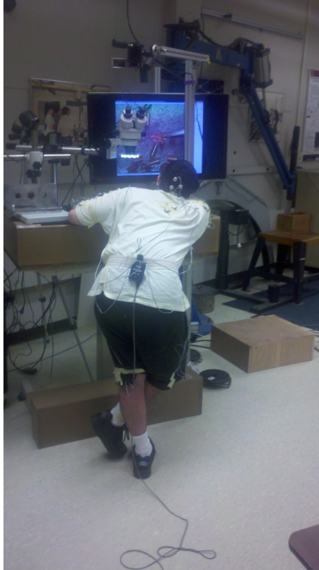
Figure 3.8: Unique posture observation while using the 3D flat-panel display. Unconstrained by microscope eyepieces, illustrated subject was observed to lean and rest upper extremity on table.
