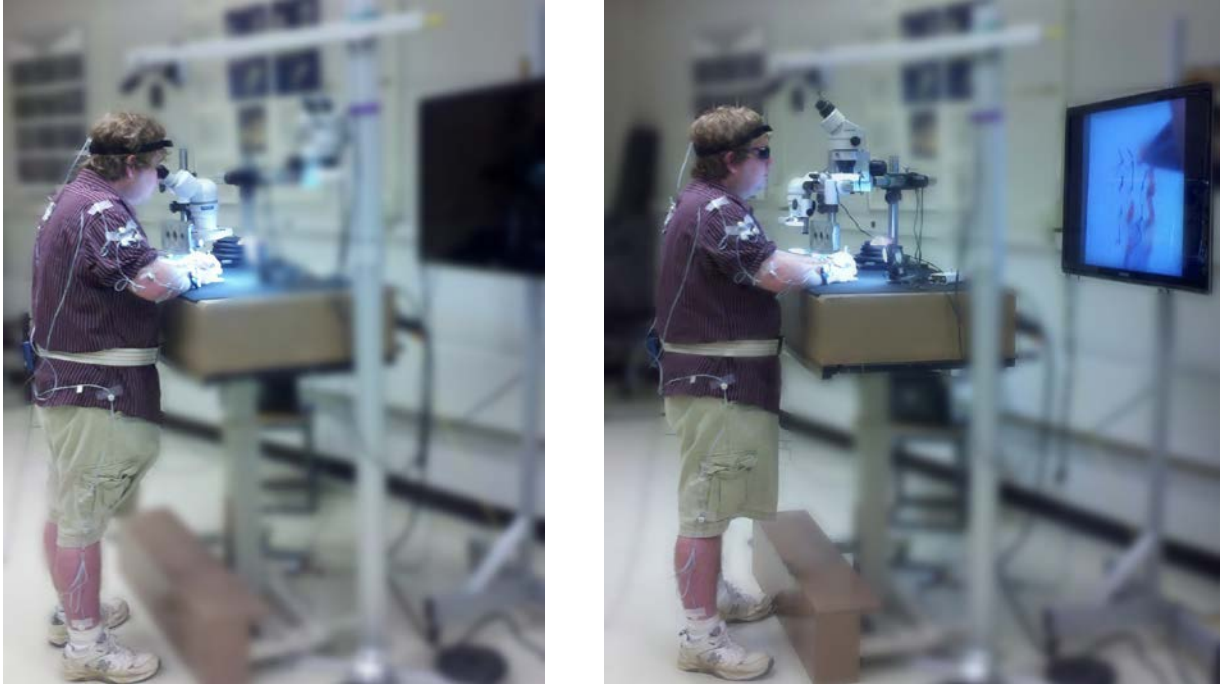
Figure 3.4: Subject performing tasks using microscope (Left) and Video 3D display (Right). Note that the set up for Video 2D display is similar to Video 3D but without the shutter glasses.
