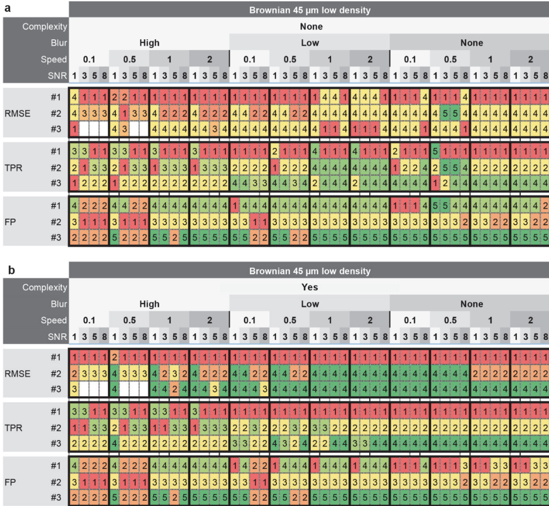
Figure 80. The top three best performing methods for each combination of properties and Brownian motion. a) 45 \mu\text{m} particles moving in Brownian motion at a low density with no particle complexity. b) 45 \mu\text{m} particles moving in Brownian motion at a low density with particle complexity. The methods are coded as follows: 1: SURF, 2: Canny, 3: Hough, 4: Otsu, 5: Threshold.
