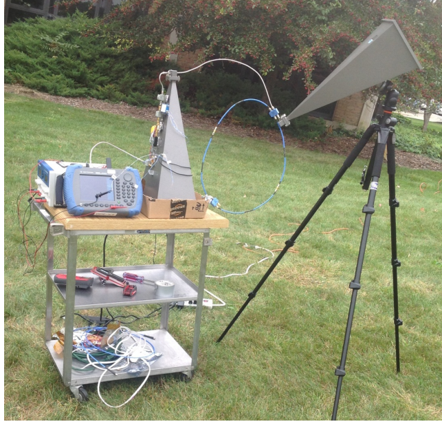
Figure 5.2: The actual implementation of the loop structure to measure the noise figure of the WiBAR.
