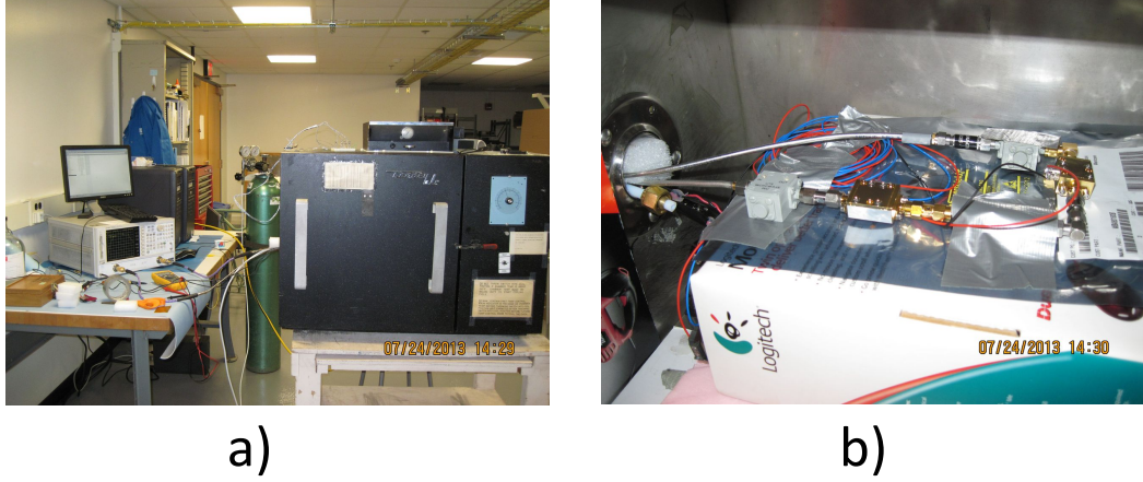
Figure 3.5: (a) The thermal setup used to characterize the system response. (b) The microwave circuit inside the thermal chamber.
