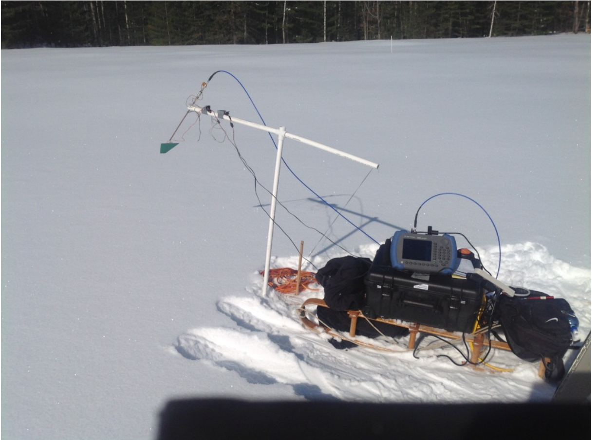
Figure 3.10: The setup used to measure the snow thickness using the second generation of WiBAR. 64cm of snow (ground-truth) is detected at University of Michigan Biological Station (UMBS) at Pellston, MI.
