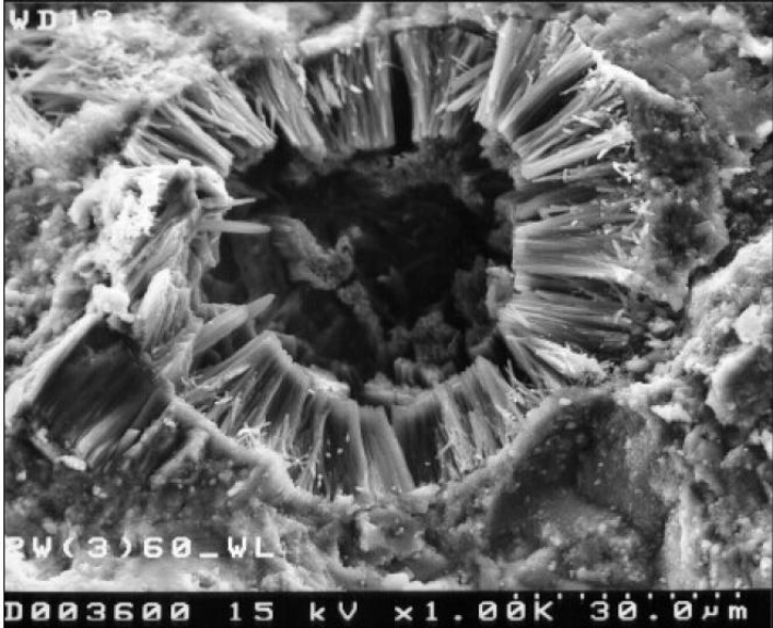
Figure 2.15 Ettringite formation in the air void (Bollmann and Stark 1996)
